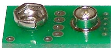
At left you can see the component side of the board with the terminal rivets before they are soldered. At right is the terminal side of the board. Note how the rivet heads are pressed all the way down inside the terminals.
